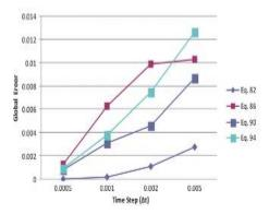
Fig. 3. Global error versus time step
