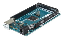
The Arduino board is a microcontroller based on the Atmega 2560 that is open-source. The processing or cabling vocabulary is handled by the board's growing environment. With their simple to use platform, these boards have reloaded the automation sector, allowing even those with little technical expertise to learn the necessary programming skills and even run the Arduino unit. These boards are used to extend interactive artifacts independently; otherwise, we'll
