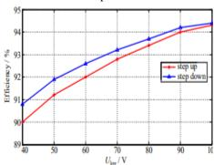
Fig. 21 Efficiencies of the proposed switched-capacitor bidirectional converter in step-up and step-down modes (U<sub>high</sub>=300V, U<sub>low</sub>=40V~100V, Pn=300W).
