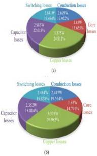
Fig. 22 Calculated power loss distributions for the experiment when U<sub>low</sub>=40V, U<sub>high</sub>=300V, and Pn=300W. (a) In step-up mode. (b) In step-down mode.
