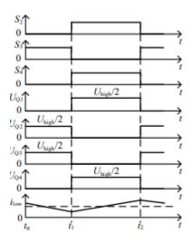
Fig. 5 Typical waveforms of the proposed converter in step-down mode.
