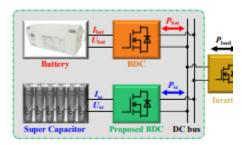
Fig. 19 Hybrid energy sources system of electric vehicles.
