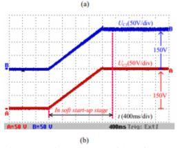
Fig. 10 Experimental results of the soft start-up. (a) The input voltage Ulow and the output voltage Uhigh. (b) The voltages across C1 and C2.
