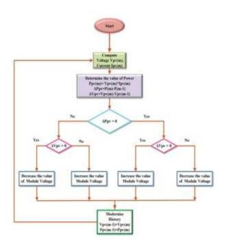
Figure 2. Flowchart of efficient control algorithm.
