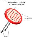
Fig 3. parts of an LDR
