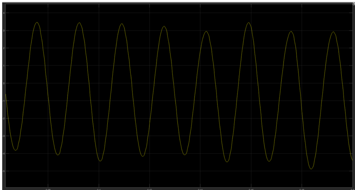
Fig 4. ripple eliminator is active with different auxiliary capacitor voltages: V_b = 600V
