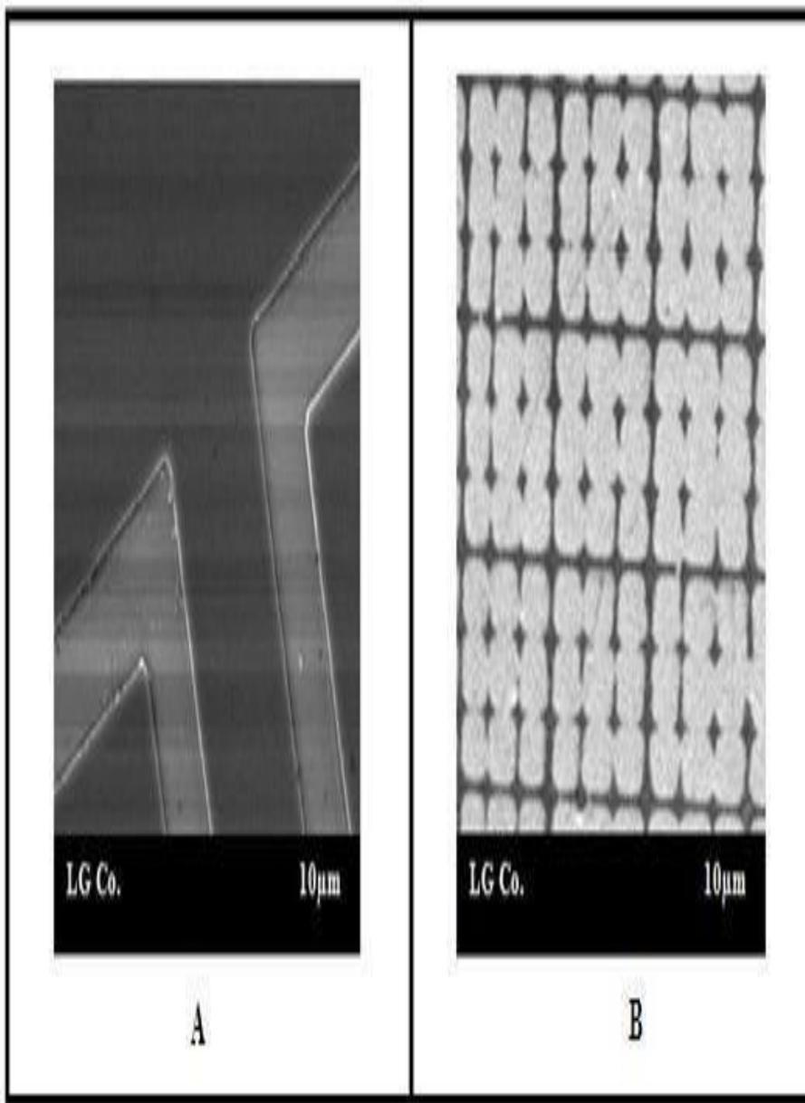
**Fig. 1. Microscopic view of MEMS: (A) Microconexions and (B) Electronic microboards to MEMS (10X)**
