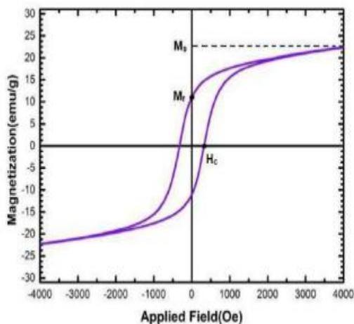
Figure 6: The hysteresis loop of CuFe2O4 nanoparticles fired at 850 OC
