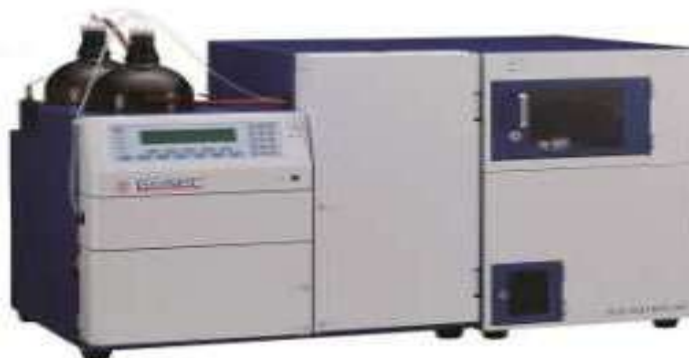
Figure 2: Instrument of gel permeation chromatography
