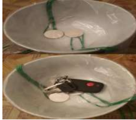
Fig: (a) Shows Piezoelectric sensor deployed in the key bowl. (b) Shows keys placed inside the key bowl.
