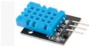
Fig – Temperature Sensor
