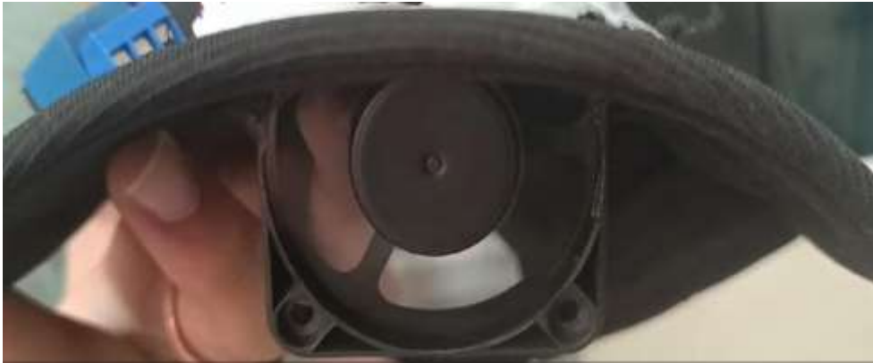
Figure 4.3: ON/OFF switch is turned on then cooling fan starts rotating
