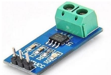
Fig. 3.3 ACS712 Hall Effect Current Sensor
