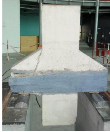
c) CP3u : Shear collapse with fabrics peeling off
