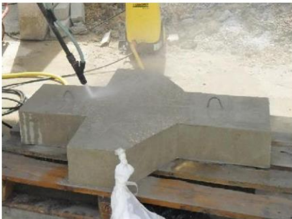
Figure 1: Surface Treatment by Sandblasting
