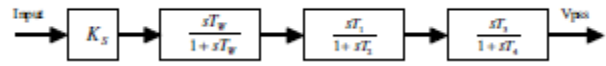
Fig.3.3: lead-lag power system stabilizer. The general equation and the used equation of the PSS is:
