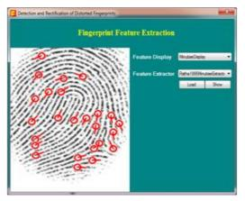
Fig.2 Minutiae Point identification with Finger-Print Bank Algorithm
