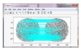
Fig.9 Minutiae-Point Matching of Training and Testing Fingerprint Image
