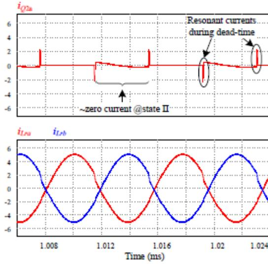
Fig. 9. Zero current characteristic of  $Q2a$ .
