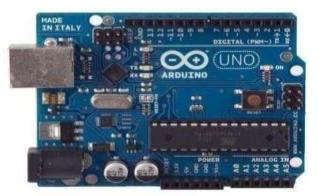
Figure5:ArduinoUNOC arrier Synchronization:
