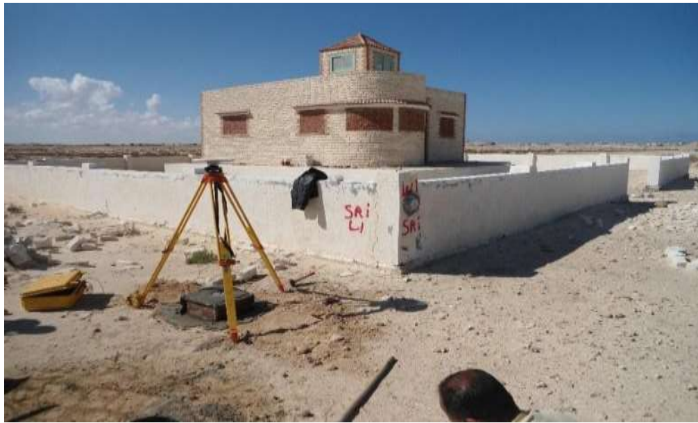
Figure 1. DGPS/Precise levelling observed stations
