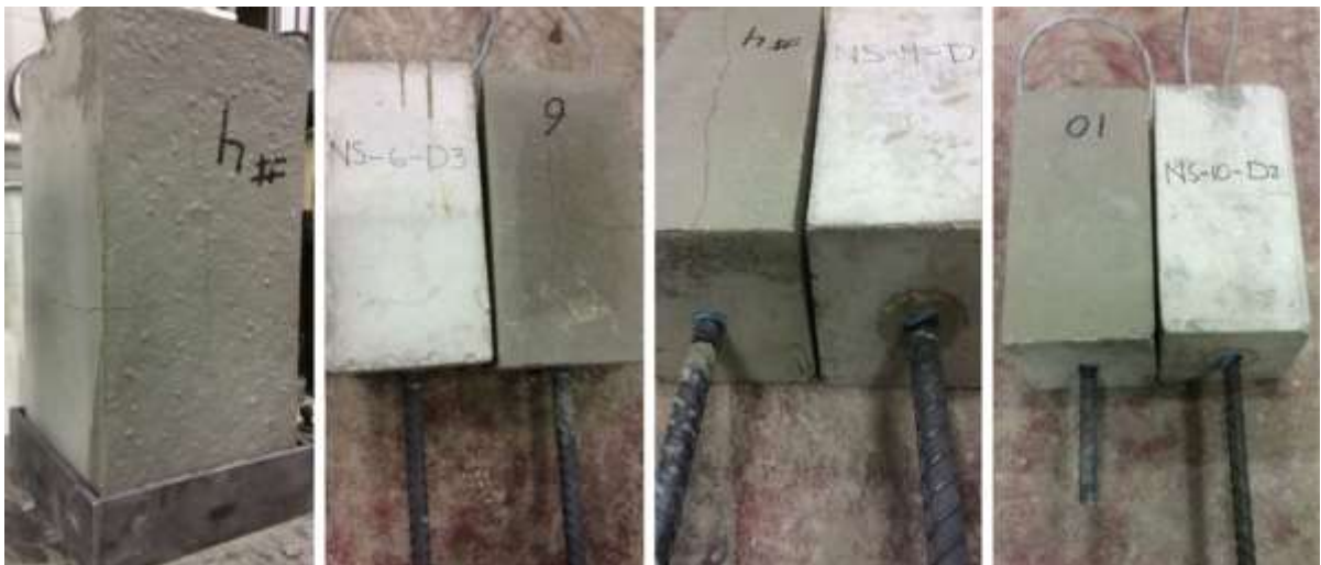
Bar Pull-out (Grouted Specimens) Splitting (Grouted/Concrete Specimens) Bar Fracture (Concrete Specimens)
