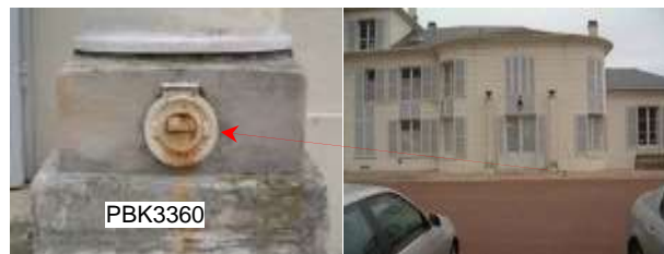
Figure 2.2.4 The NGF-Lallemand leveling point on the wall of the Nouveau Pavillon building of BIPM and is numbered P.B.K3-360 with its value 66.0612 m in IGN69. The last measurement visit was in 1968 by the IGN. This is the back-up point.
