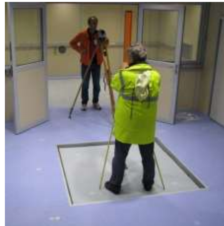
Figure 2.2.2 Site WB and the gravity-stations of which 6 are leveled (W1, W2, W11, W14, W15 and W18). The top surface of the pillar W1 is 7 cm lower than surrounding ground surface (dimensions in cm). A leveling between W1 and W2 is undertaken
