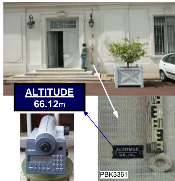
IGN69. The leveling measured and computed
