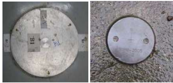
Figure 2.2.3 Two kinds of benchmarks on the indoor (left B1) and the outdoor (right C2) gravity stations
