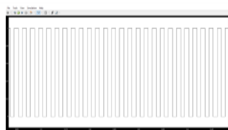
Fig 4.1 and 4.2 shows gate pulses generated for IGBT's operation by using HBCC pwm method for AC chopper
