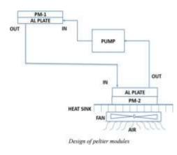
Design modifications were made to enhance cooling efficiency and prevent heat damage. Two Peltier modules are used instead of one. addressing previous drawbacks. A DC pump facilitates heat transfer from Peltier Module 1 to Peltier Module 2 through water. The heat is then removed through a heat sink, resulting in simultaneous cooling of Peltier Module These modifications optimize cooling performance within the system.
