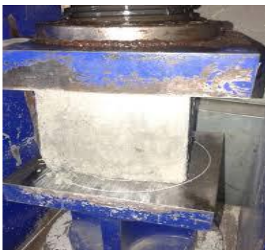
Fig 3.5.1 Compressive strength testing machine
