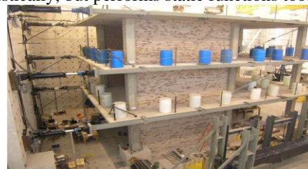
Figure 1 : Test Structure with Infill Walls
