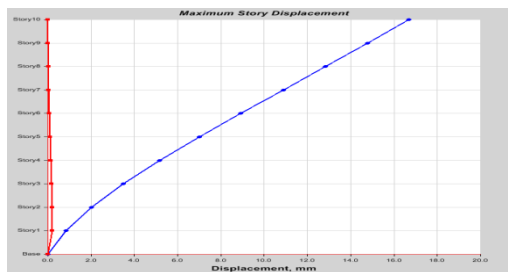
Figure 15: Storey displacements of structure with infill walls and without soft storey for Push X using pushover analysis
