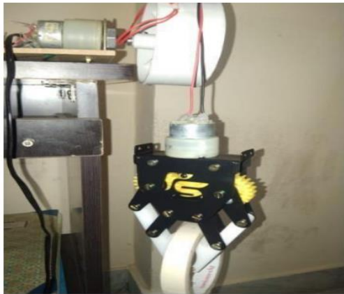
FIG 6 OBJECT PICK UP WITH HELP OF GRIPPER
