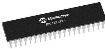
Fig.10 PIC Microcontroller (PIC16F877A)
