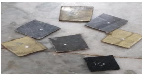
Figure 28 AFTER TESTING OF HARDNESS SPECIMENS
