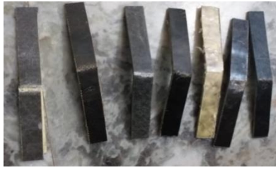
Figure 26 AFTER TESTING FLEXURAL SPECIMENS
