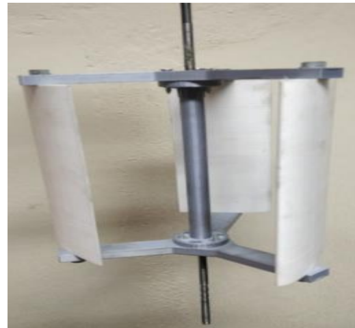
Figure7: shows the comparison of twisted CL/CD and twisted blade assembly
