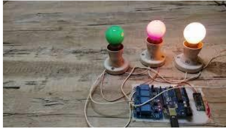
Fig 7. Hardware Implementation of Home Automation System
