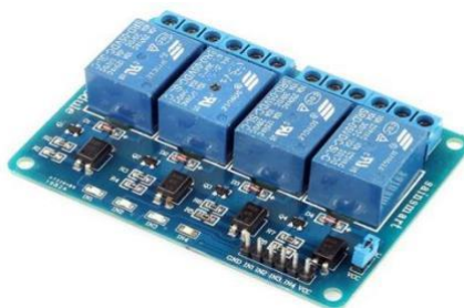
Fig 3. Four channel Relay Module
