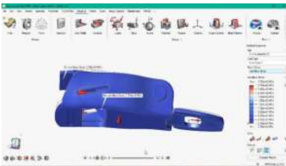
Figure 12 Von Mises stress for AISI 304 S.S
