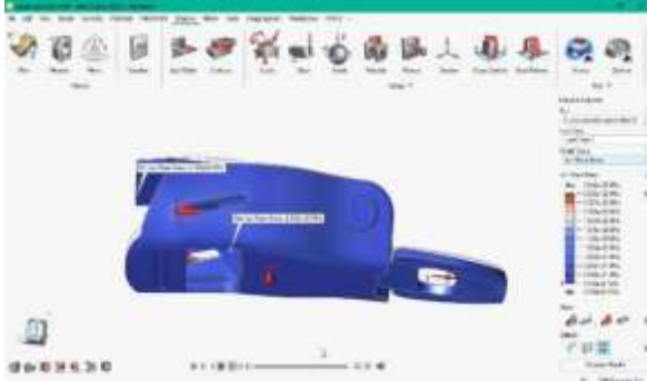
Figure 14 Von Mises Stress for CF T700
