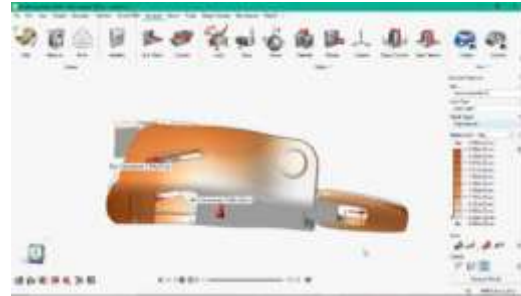
Figure 11 Displacement of AISI 304 S.S
