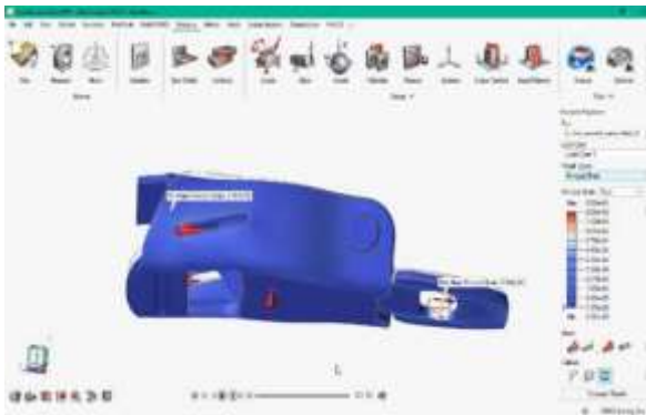
Figure 16 Principal Strain for CF T700
