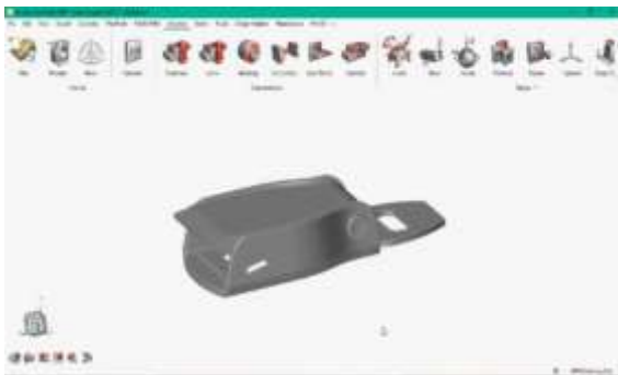
Figure 8 Assembly File in Altair Inspire
