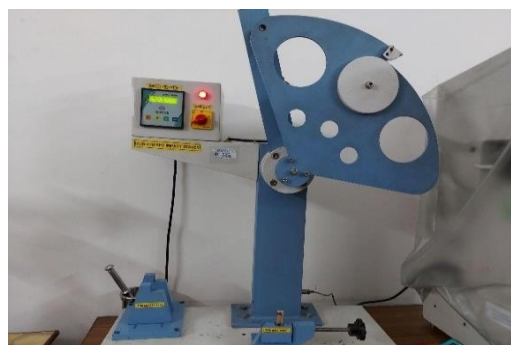
Figure 7. Izod impact test equipment
