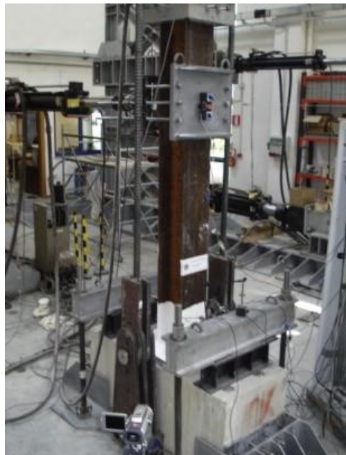
Figure 2. Column base connection test setup [9]
