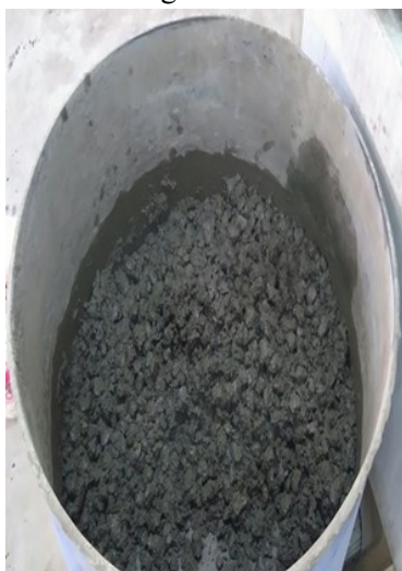
Figure 3.4 Mixing of Solution to aggregates and glass fibres
