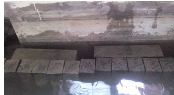
Figure 3.6 Curing of Specimens
