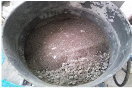
Figure 3.2 Mixing of glass fibres, Cement, coarse & fine aggregate
