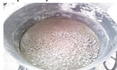
Figure 3.1 Mixing of coarse aggregate and fine aggregate
