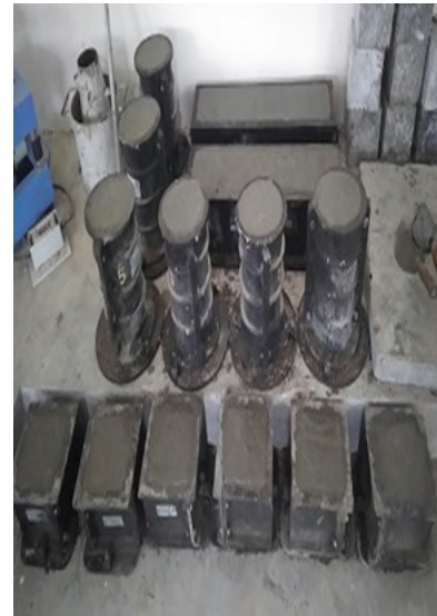
Figure 3.5 Casting of M30 grade Glass Fibre Reinforced Concrete
