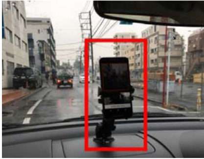
Fig. 1. Installation setup of the smartphone on the car. It is mounted on the dashboard of a general passenger car. Our developed application can capture a photograph of the road surface approximately 10 m ahead, which indicates that this application can photograph images while traveling on the road without leakage or duplication when the car moves at an average speed of about 40 km/h (about 10 m/s) if photographing every second. In addition, it can detect road damages in 1.5 seconds with high accuracy (see Section 5).
