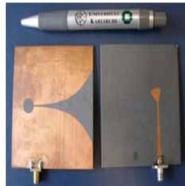
Fig. 6. Aperture coupled Vivaldi antenna. (Left) Top view; (right) bottom view with feed line. Substrate size 75 _ 78 mm 2 .
