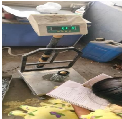
Figure-9: Specific gravity test of coarse aggregate
