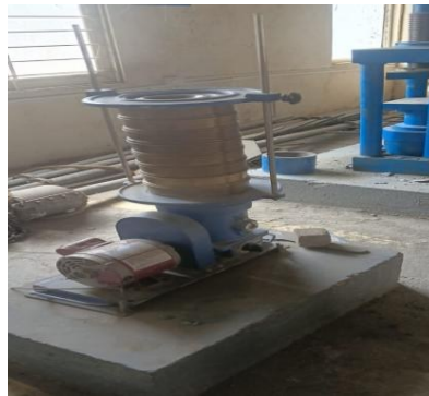
Figure-11: Sieve analysis of fine aggregate
