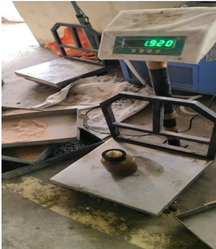
Figure-10: Specific gravity test of fine aggregate
