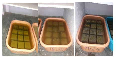
Immersion of Specimens in Acids and Sulphate
