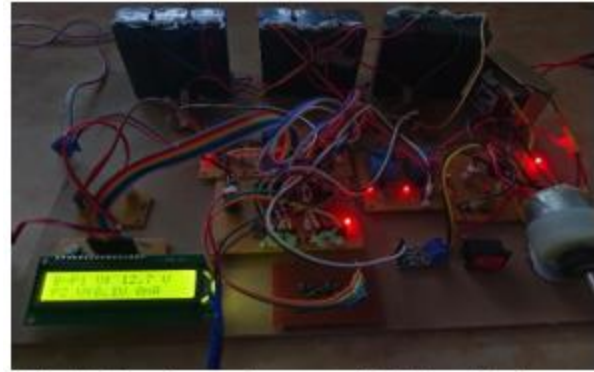
Fig 5. Experimental set up of BMS with charge monitoring and fire protection
