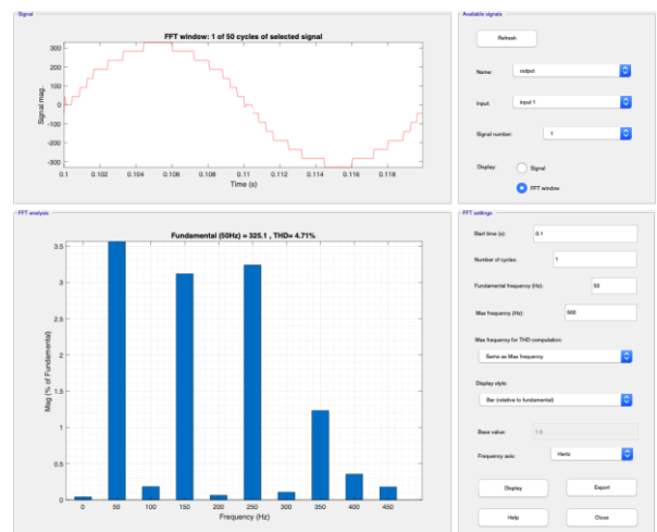
Figure 8: FFT analysis of 15 level inverter's output voltage
