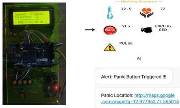
Fig.4. Output of panic alert system
