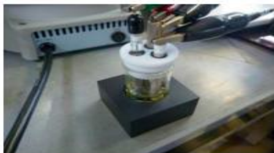
Fig. 1. Fabrication of amino group terminated SAM on the Au electrode; immersion set-up of the electrode (left) and surface of the electrode immersed overnight (right).
