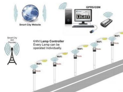
Fig 1. Street light controller with wireless technology
