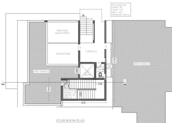
Fig 3.4 Stair Room Plan
