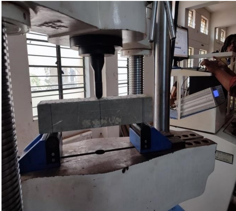
Figure 5. Flexural Strength Test equipment
