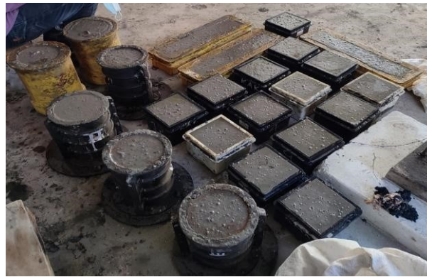
Figure 2. Casting of specimens
