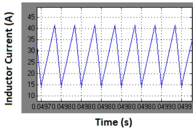
Fig.5 Simulated response of inductor current for modified high gain converter using APICs ( $V_{in}=40V$ ,  $R=50\text{ Ohm}$ )
