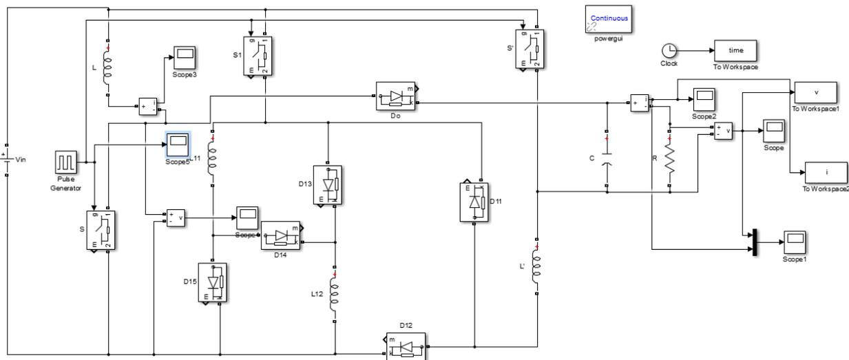
Fig.3 Working of the modified high gain converter using APICs, (a) during on time period of switches and during off time period of switches
