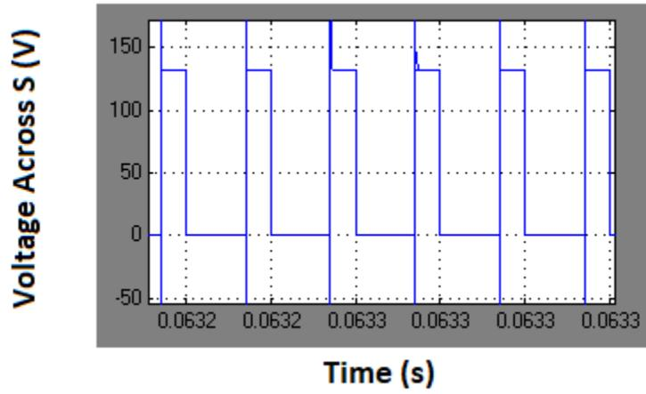
Fig.6 Simulated response of voltage across the switch S for modified high gain converter using APICs ( $V_{in}=40V$ ,  $R=50\text{ Ohm}$ )
