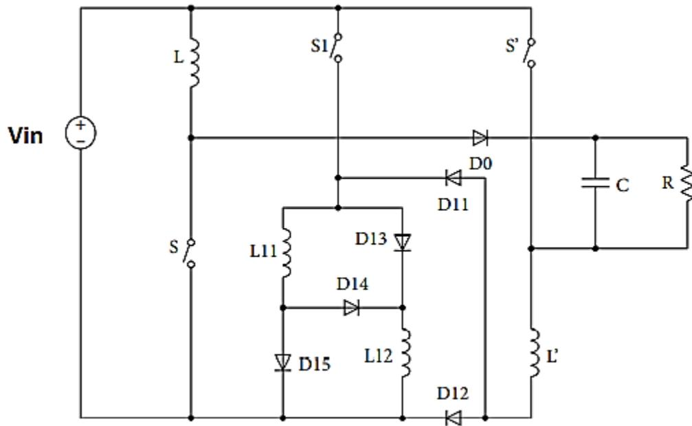
Fig.1 Circuit diagram of the modified high gain converter using APICs
