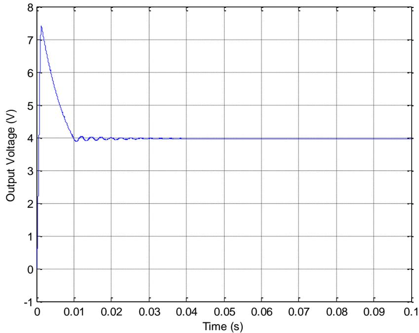
Fig.9 Simulated output current response for modified high gain converter using APICs ( $V_{in}=20V$ ,  $R=50\ \Omega$ )
