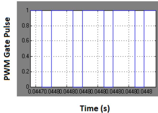
Fig.4 Simulated response of PWM gate pulses of switches for modified high gain converter using APICs ( $V_{in}=40V$ ,  $R=50\text{ Ohm}$ )
