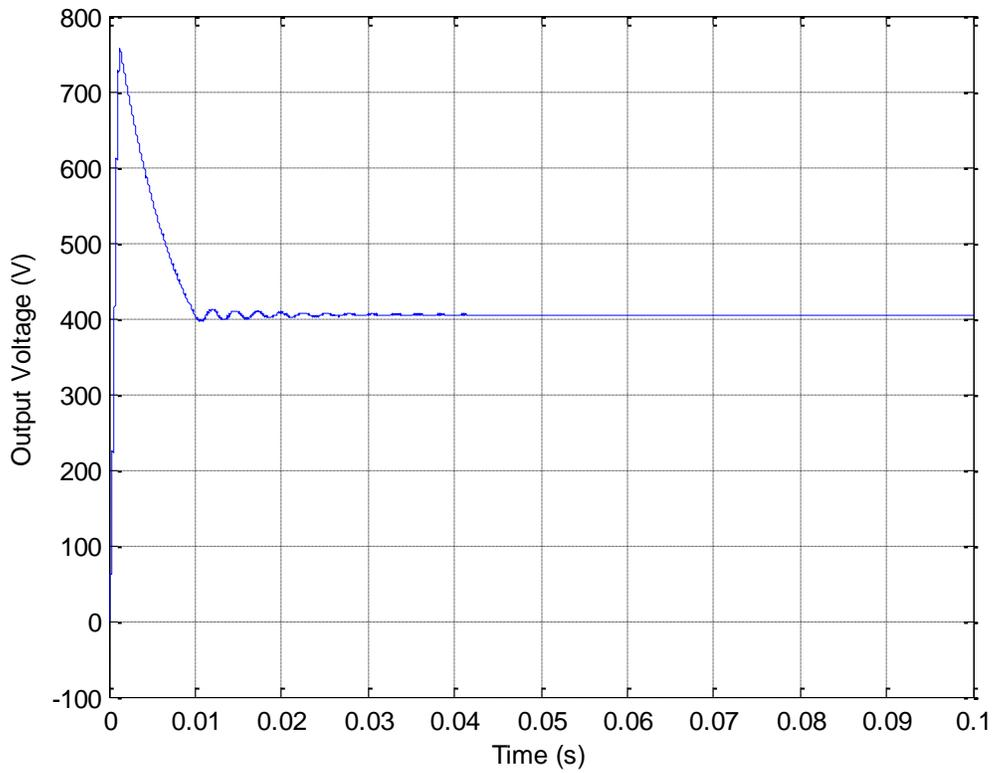
Fig.7 Simulated output voltage response for modified high gain converter using APICs
