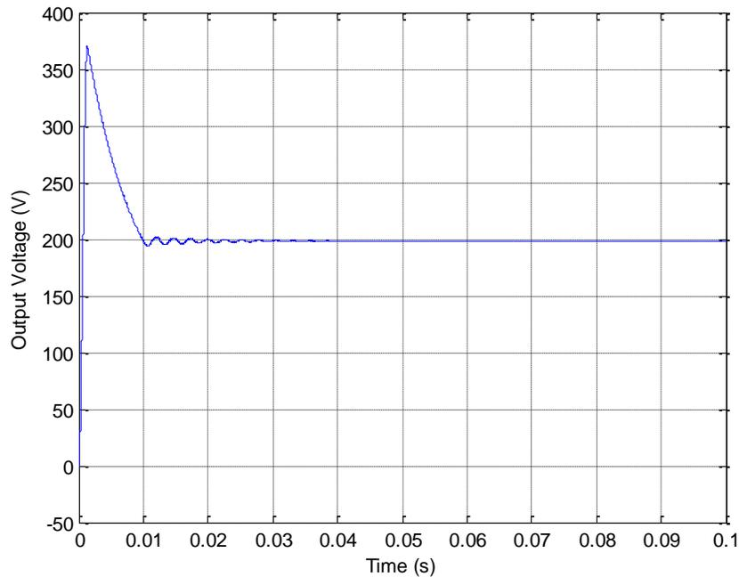
Fig.10 Simulated output voltage response for modified high gain converter using APICs ( $V_{in}=20V$ ,  $R=50\ \Omega$ )
