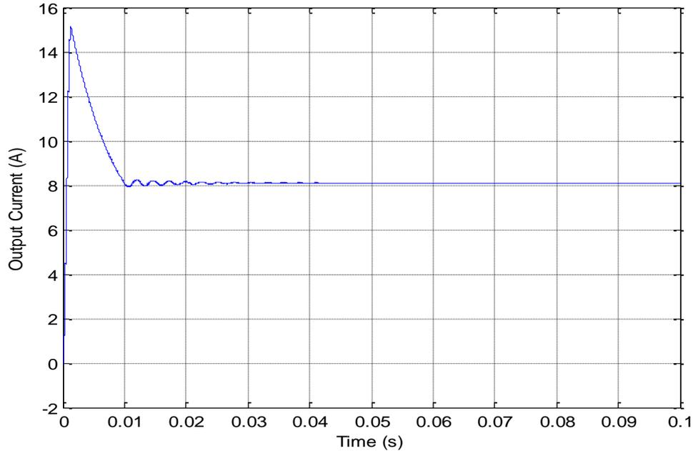
Fig.8 Simulated output current response for modified high gain converter using APICs ( $V_{in}=40V$ ,
